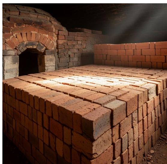
Figure 3: Standard bricks in their molded form (in a rectangular shape) after firing in a traditional clamp kiln.
